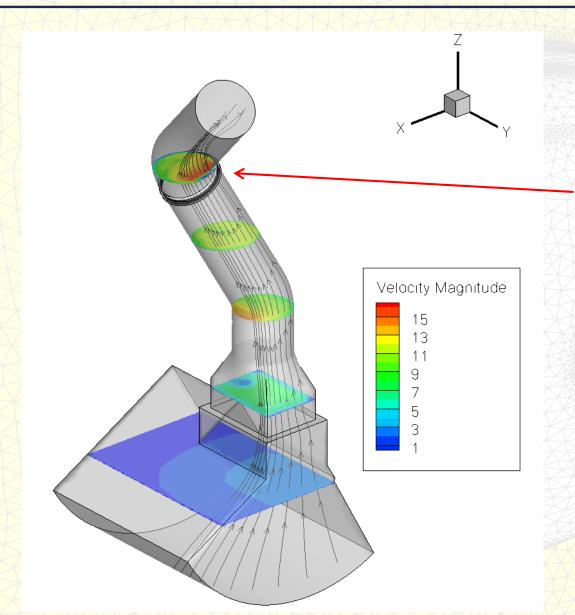
Flow separation causing problems in compensator
