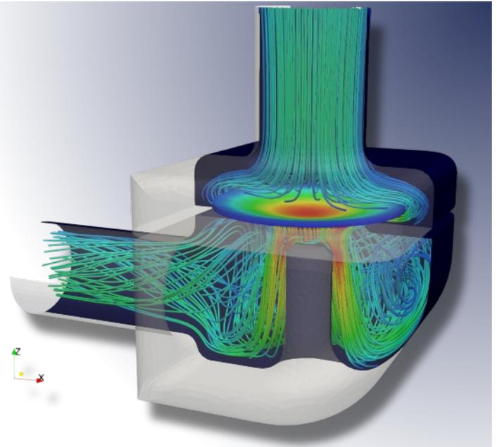
Valve case: Elastic membrane deformation by increasing pressure
